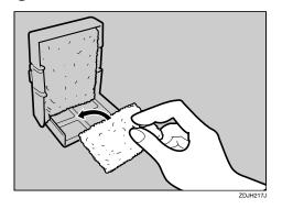
Insert the dustproof filter cover into the upper left area of the printer.
