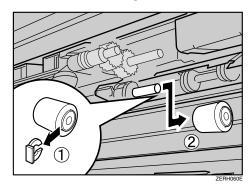
Hold the new paper feed roller C with its gear towards the shaft. Insert it into the rear shaft so that the roller gear interlocks with the shaft gear (1). Lock the roller with the stopper (2).
