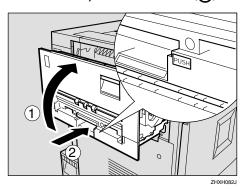
If you removed the external tray in step [4], reattach it to the printer. Insert the hooks of the external tray into the printer slits, and then lower it toward you.
