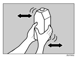
Holding the toner cartridge with the metal contact area in front, insert in the direction of the arrow.
