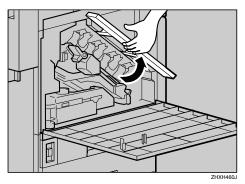
The photoconductor units are installed as shown. Starting from the upper left, the units are attached in the order of black (K), yellow (Y), cyan (C), and magenta (M).
