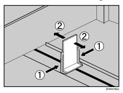
Align all four sides of the paper stack, and then load it in the tray.
