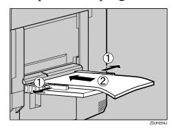
Adjust the side guides to fit the paper width.
