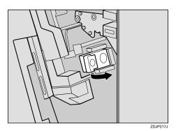
3 Open the cartridge face plate to unlock it.
