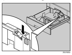
2 Press the side guide green lever (1), adjust the position of the guide by moving it in the direction of the arrow (2).
