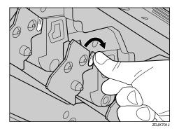
2 Hold the hook down, grip the green areas at the top and bottom of the photoconductor unit, and then slowly pull the unit out until you can see the entire green handle.
