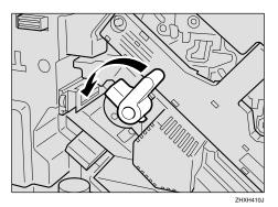
4 Loosen the two screws fastening the inner cover, using the provided screwdriver.
