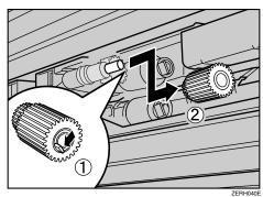
Remove the stopper from paper feed roller B (1), and then remove the roller (2).
