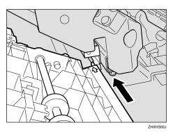
Refasten the duplex feed unit using the provided screwdriver. Use the screw removed in step 4.
