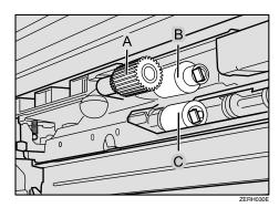
While pushing the pin of paper feed roller A outwards (1), remove the paper feed roller (2).
