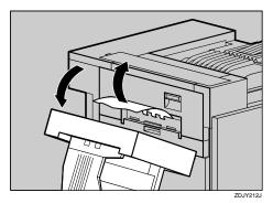
Slowly raise the duplex reversal unit and insert until it clicks into place. Raise the left cover, and then close it securely by pushing the area labeled "PUSH".
