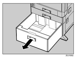
With the print side down, align all four sides of the two paper stacks, and then load them next to each other in the tray. Each side has a limit of 1,000 sheets.
