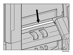
Wipe around the registration roller by turning it and applying a soft damp cloth.
