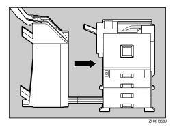
The 2 tray finisher is reattached to the printer.
