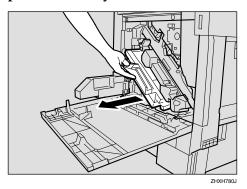
6 Hold the duplex feed unit using both hands, place it on the vertical rail, and slide it straight out.
