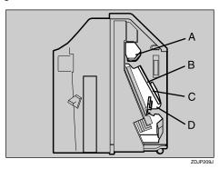
Check area A of step 4. Lift the lever (1), and then while holding it up with your hand, slowly pull out the misfed paper.
