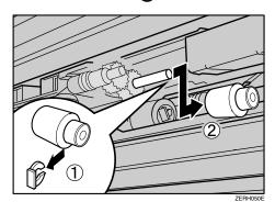
Remove the stopper from paper feed roller C (1), and then remove the roller (2).
