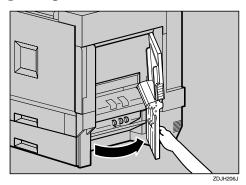
Move the blue lever up and down to feed the misfed paper, and then slowly pull out the paper.
