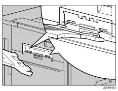
If the duplex unit is installed, close the duplex reversal unit.
