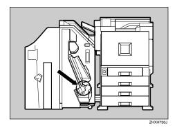
**2** Remove the cartridge by pulling the green knob in the direction of the arrow.
