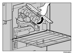
The development units are installed as shown. Starting from the upper left, the units are attached in the order of black (K), yellow (Y), cyan (C), and magenta (M).
