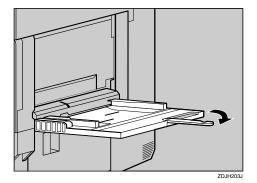
2 Slide the side guides outward (1), and then load paper print side up, until it stops (2).
