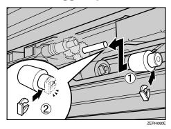
Hold the new paper feed roller A with its pin towards you (1). Insert the roller onto the front shaft until it clicks into place (2).
