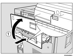
If you removed the output tray in step 3, reattach it to. Insert the hooks of the output tray into the printer slits, and then lower it toward you.
