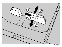
Adjust the end guide according to the size and orientation of the paper by gripping both edges of the guide (1), and then moving it in the direction of the arrow (2).
