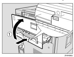
If you removed the external tray in step 4, reattach it to the printer. Insert the hooks of the external tray into the printer slits, and lower it toward you.
