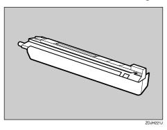
2 Hold the photoconductor unit, and remove the adhesive tape at the tip of the unit.
